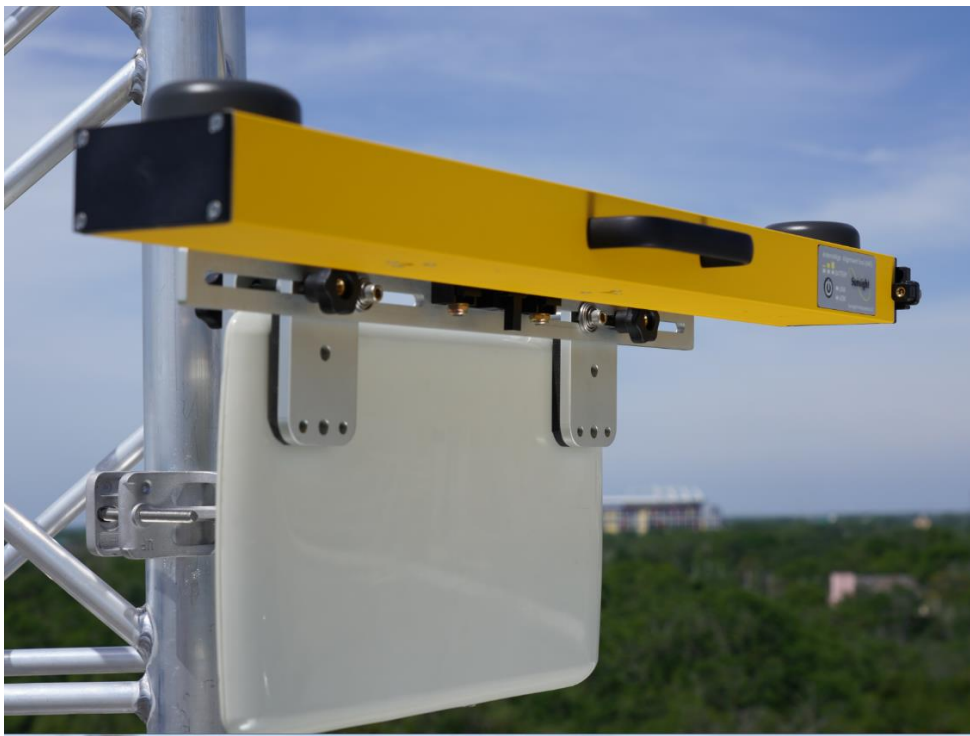
Flat Panel Antenna Mount on Radwin JET Antenna (with AAT)
